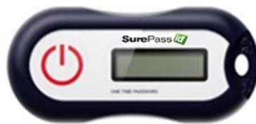
Button on front, Event-based (HOTP) Token 2-3/8" x 1" x 3/8"
